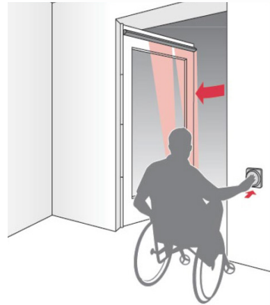
AUTO-IR Presence Sensor and Door Activator 48", Length Field-Adjustable
