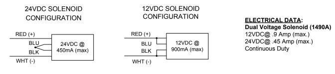
PR1000 Input Voltage: 12/24 VDC/AC (+/-10%). DC voltage is recommended for optimal performance
