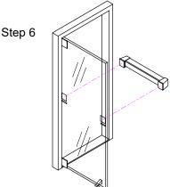
Press and hold bar firmly in place against the glass door for approximately 3 minutes until bar is secured to door
