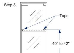
Using tape, mark bar location on outside of glass door.
