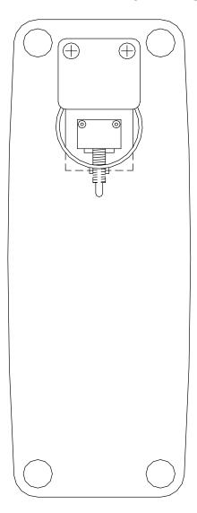
REMOVE TWO TOP ASSEMBLY SCREWS PLACE SWITCH ASSEMBLY AS SHOWN AND FASTEN SCREWS.
