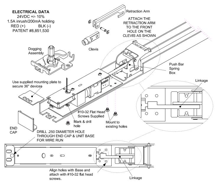
When retrofitting to existing vertical rod devices, adjustment of the rods is required for proper operation of the Electric Latch Retractor. Once the unit is properly installed, energize it so the latch is dogged down, then reconnect the vertical rods to the device and make the proper adjustments.
