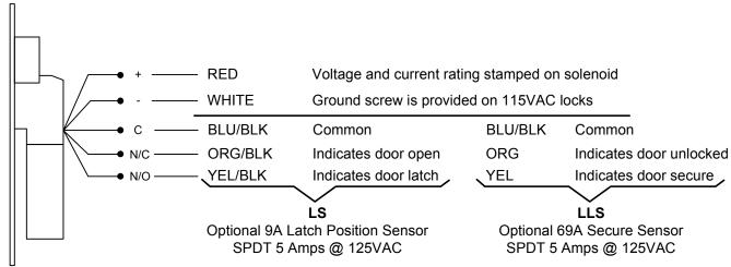
\* Wiring assignments for the optional SC-10 cable with socket connectors are the same
