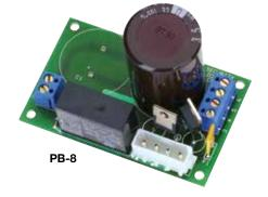
Modules may be ordered with or without power supplies. Different function modules may be used in the same power supply or cabinet. Contacts: 2.5 Amps tretive, 5 Amps resistive @ 30 VDC unless specified otherwise.
