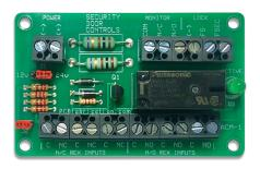
Door control relay modules ensure compatibility of access hardware components and simplify system installation and troubleshooting. Modules may be ordered with or without power supplies. Different modules may be specified for one power supply.
