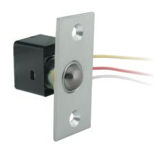
**SDC's DPS series sensors employ electromechanical ball switches** to provide a cost-effective means of monitoring door position status (DPS). DPS monitors the current position of the door, open or closed. DPS switches change state when the door is opened or closed. Installed in the edge of the door frame, DPS switches are wired into remote devices, typically alarm panels or door controllers, to notify facility management of a change in state - aiding in an access control system's integrity.
