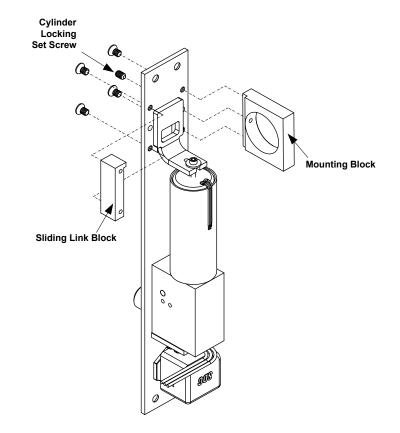
Make sure the sliding Link Block is positioned properly
