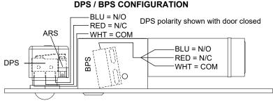
BPS polarity shown with bolt retracted.
