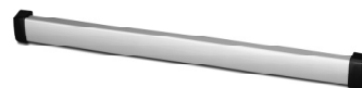
PSB560 Request-to-exit touch sense non-latching bar that will activate the Exit Check® when slight pressure is applied to the bar. For doors without latching.
