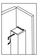
**CAUTION:** The lock body must be held in place until secured with mounting screws. Secure socket head screws provided inside the housing at each end. Start screws into threads carefully to avoid stripping the threads. Check alignment and tighten screws. Pull wires through frame, mounting plate and magnet housing
