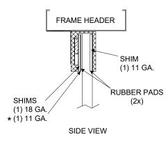
\* Second 11 GA. Shim Not Required For 5/8" thick Door Installs.
