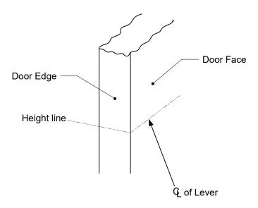
2. Place template on edge of door as shown and align lever centerline with marked height line on door. Check the chart for drilling trim holes on template and only mark holes for lock function being installed.
