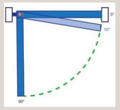
Doors shall close from 10 degrees (latch-check) to fully closed in not less than 1.5 seconds
