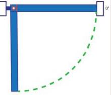
**Exception:** When push-pull activation is used, the door shall remain at the fully open position for not less than three seconds.
