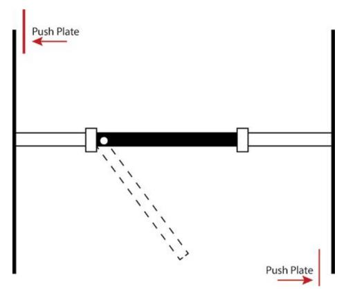
Knowing Act: Consciously initiating the powered opening of a low-energy door using acceptable methods, including: wall or jamb-mounted contact switches such as push plates; fixed non-contact switches; the action of manual opening (pushing or pulling) a door; and controlled access devices such as keypads, card readers, and key switches.
