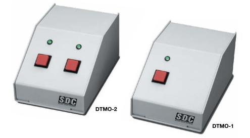
The SDC Mini Desktop Consoles provide an economical method of controlling one or two doors. They are available in four switch configurations with Tri-Color LED indicators. When used with a door status or lock status sensor the LED's allow monitoring of door and lock modes. The switches can provide an On / Off function or momentary access control for electromagnetic EMLocks, Shear Locks, Bolt Locks, Delayed Egress Systems, Electrical Exit System, or Electric Strikes.
