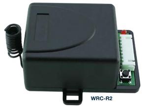
SDC's WRC Series 2-Channel wireless transmitter/ receiver solution is specifically designed to be used as a receptionist button or remote release for single or dual door access control applications. Receiver has the capacity to learn up to 30 fixed transmitter codes using the onboard learning button and status LED.
