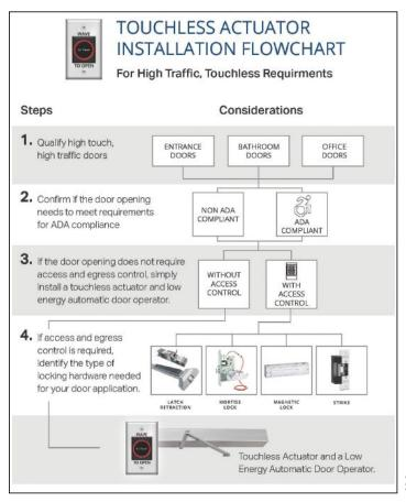
touch only, chances are you can pair the actuator with the existing electrified locking hardware and you're finished.
